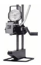
These tests measure the depth or area of an indentation made by an intender with a specific force applied for a specific time.
