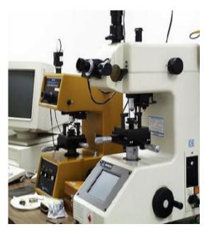
Micro hardness test involves using a diamond indenter to make a micro indentation into the surface of the test material; the indentation is measured optically and converted to a hardness value.
